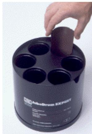
[Inserting Film Into the Expert Drum #3010]
